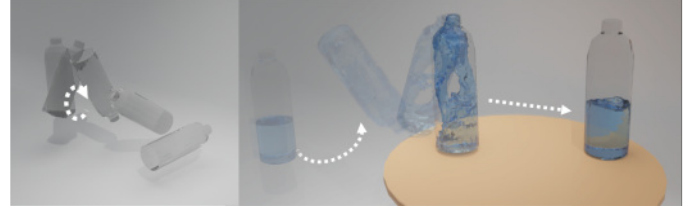
Fig. 6. (Left) Demonstration of fluid-rigid coupling: An empty bottle with the same optimized initial linear and angular velocity in Fig 5. Without fluid-rigid interaction, the bottle spins very fast. (Right) Based on the optimization result of the first stage where we only consider fluid-bottle coupling, we further consider the bottle-table collision stage to fine-tune the initial velocity of the bottle to make it able to stop and stand stably on the table.
